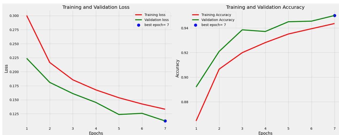
FIGURE 3. Training and validation performance metrics of the LSTM model: (a) Training and Validation Loss, (b) Training and Validation Accuracy.
